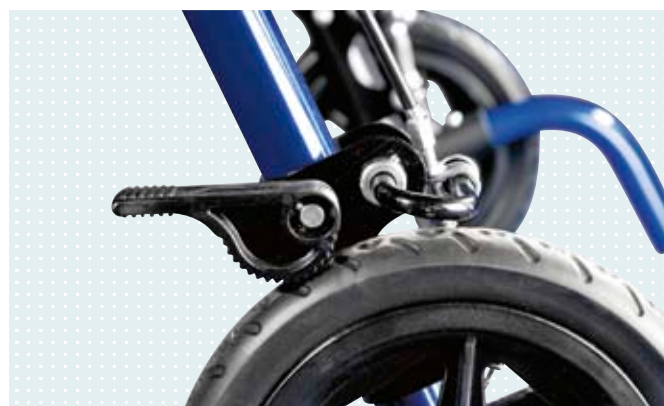
▸ Reverse-roll locking devices on the rear wheels (can be activated and deactivated)
