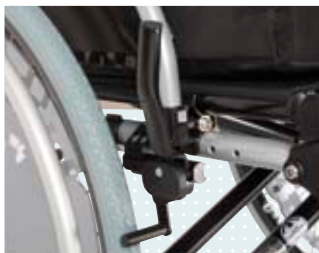
• Wheel lock lever extension
